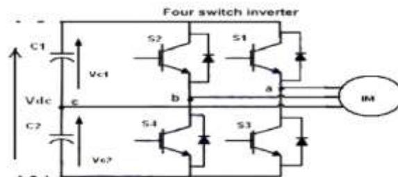
Fig 4: Two-leg three phase inverter fed IM
