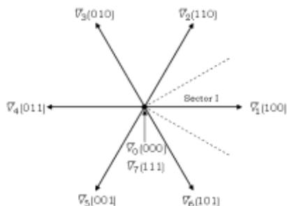
Fig2: Representation of six active voltage vectors and zero vectors
