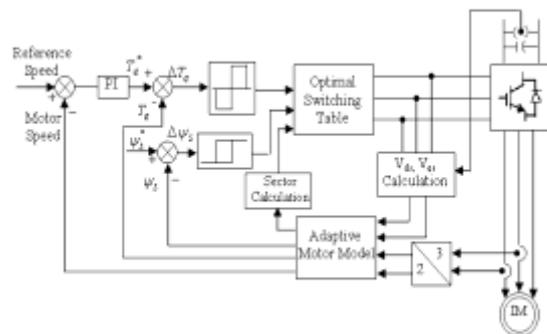
Fig 1: Conventional DTC Control Scheme for IM
