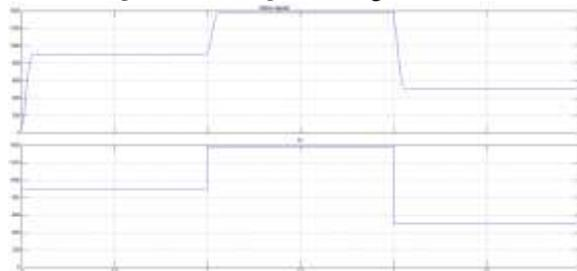
Fig16: Upper fig: Actual Rotor Speed & Lower fig: Reference Speed Using FLC
