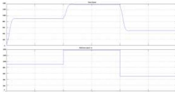
Fig15: Upper fig: Actual Rotor Speed & Lower fig: Reference Speed Using PI Controller
