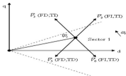
Fig3: Reference stator flux representation in sector-I
